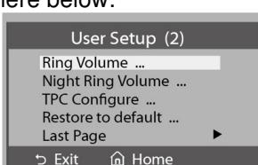
The RING VOLUME option allows to adjust the volume of the played melody in day time (6:00 to 18:00). This monitor allows to set a different volume for calls during night time (18:00 – 6:00) with NIGHT RING VOLUME option. Setting volume to 0 value,
